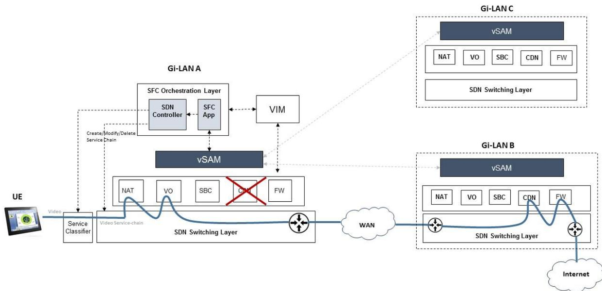
**Figure 4. Gi-LAN service-chaining adaptation for Video service-chain**
