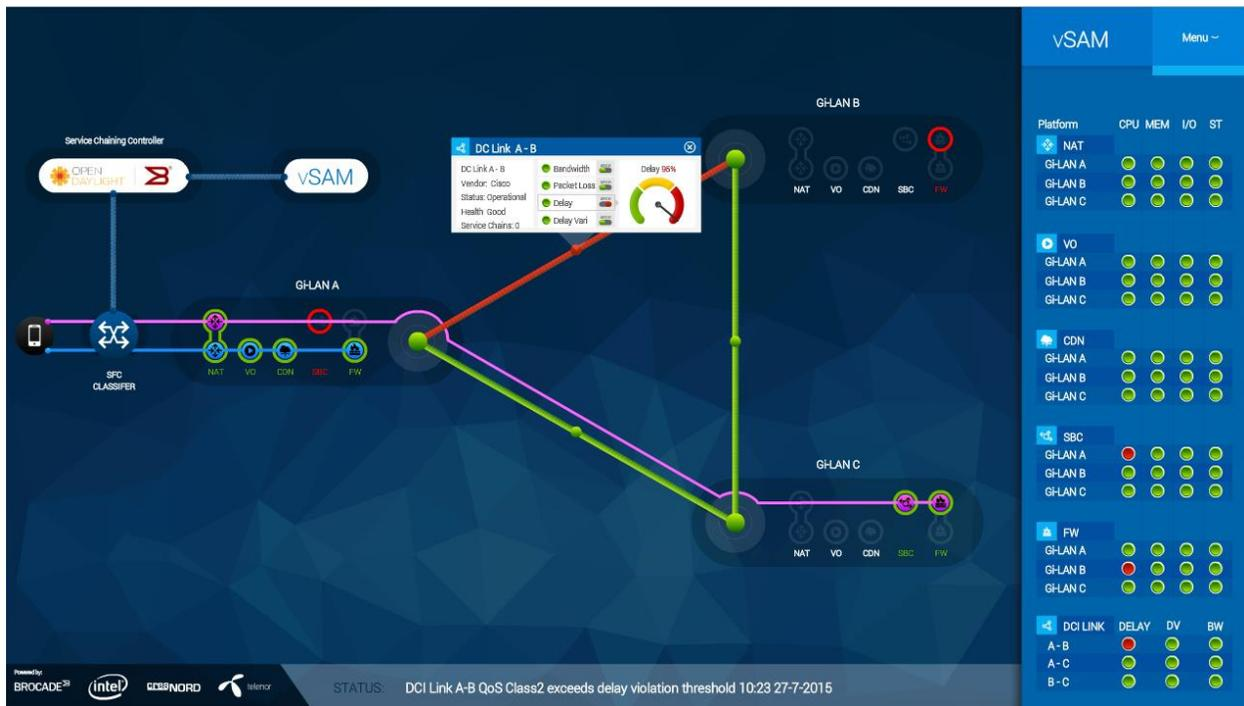
Figure 6. GUI illustrating Gi-LAN service-chaining adaptation for WAN underlay overload condition
