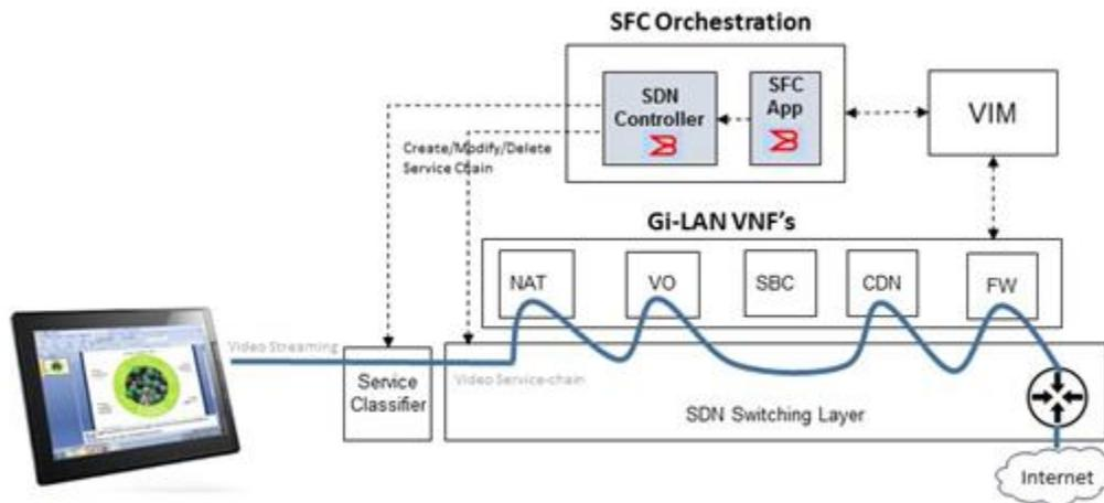
**Figure 3. Gi-LAN service-chaining for video streaming request from UE**
