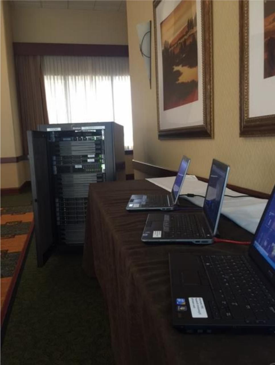
Picture #3 – demo setup HW showing details of the rack with controller, storage and compute nodes for demo clouds in the background, and three laptops used to show what happens to streamed video sessions in each of the three availability modes (FT, HA, and GA) that were demonstrated as part of the PoC.
